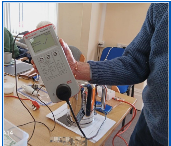
PAT testing unit showing positive result on group member's kettle
