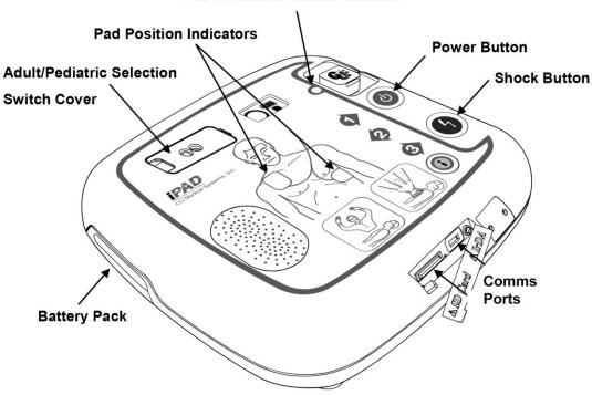
**Power Button** Turns the device on/off. Green LED lit
