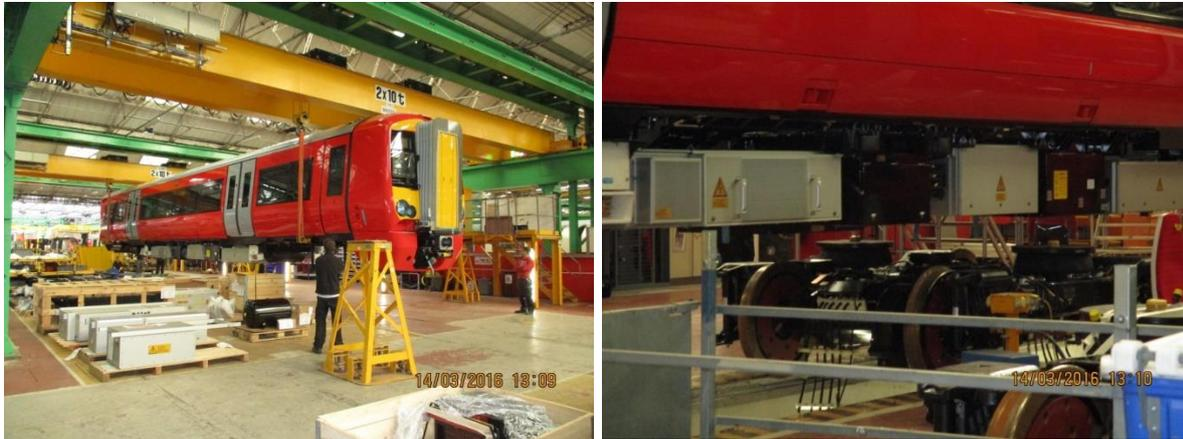
A completed carriage being lifted through the workshop and placed on two sets of wheels.
