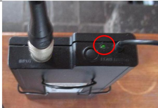
**Unipac Transmitter instrument and microphone controls, allow you to set the optimum settings for either microphone or an instrument.**
