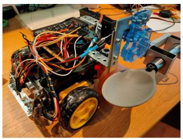
A four-wheel drive buggy giving a tiny turning circle, and thereby enhanced manoeuvrability. Bob is used for the Maze challenge where it acquires positional information from 3 narrow beam laser distance measurement sensors and is adapted for the egg and spoon challenge
