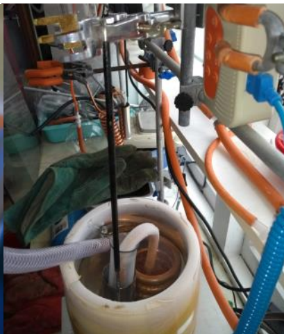
Liquid oxygen being condensed in a copper coil immersed in liquid nitrogen
