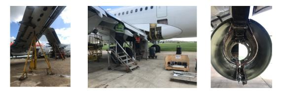
We moved to the outside to see a couple of airliners in the first stages of disassembly. The first thing to come off are the engines, which are overhauled and returned to service. A new engine costs in the region of £35 million. A second hand one is worth about £3 to £5 million, a great incentive to bring them back to service.
