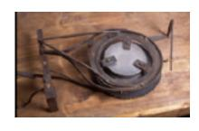
The reflector was cast in the basement of the house from an alloy of copper and a high percentage of tin. The mould was made from a mixture of horse manure and plaster. The cast reflector then required weeks of hand polishing. To speed this up, he also invented a polishing machine.
