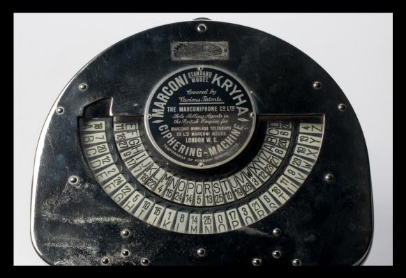
Developed in the 1920s, the Kryha was a clockworkdriven mechanical device for encryption and decryption
