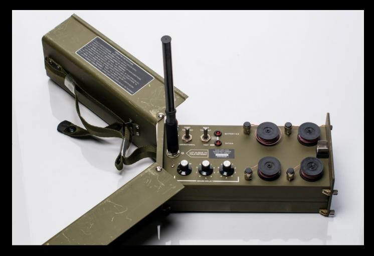
When activated, this device would jam all radio communications around it then self-detonate after its cycle was complete
