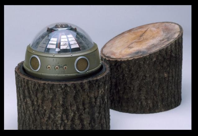
This solar powered concealment device was used to intercept radar & communications signals US intelligence designed the device to look like a tree stump and then planted it in a wooded area near Moscow A bug inside eavesdropped on radar and communications from a nearby Soviet airbase
